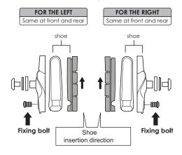
Tighten the fixing bolt. Tightening torque: 1-1.5 Nm.
