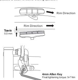
Note - Road brakes allow the angle of contact between the shoe and the rim (toe-in) to be adjusted. Adjusting the tore-in makes it possible to obtain smoother braking operation.
